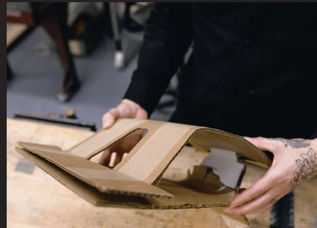
An early cardboard prototype of Steelcase Karman's weight-activation mechanism.
